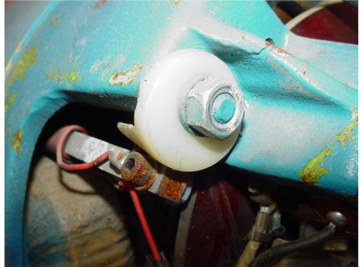
Added Magnetic Probe Next to Stator Winding
